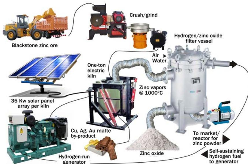
Schematic of the Blackstone Mine ore processing circuit
