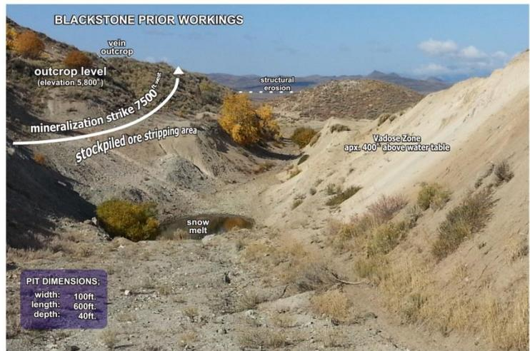
Exploratory drilling at the Blackstone established the minimum depth of the zones to be 400 feet.
